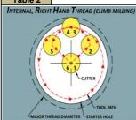
Step 1-2: Cutter moves into position Step 2-3: Cutter engages part with arcing tool nath while "7" feeds up
