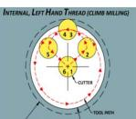
Step 1-2: Cutter moves into position Step 2-3: Cutter engages part with arcing tool path while "Z" feeds down
