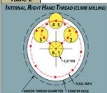
Step 1-2: Cutter moves into position Step 2-3: Cutter engages part with arcing tool nath while "7" feeds up from bottom
