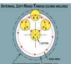
Step 1-2: Cutter moves into position Step 2-3: Cutter engages part with arcing tool path while "Z" feeds down from top
