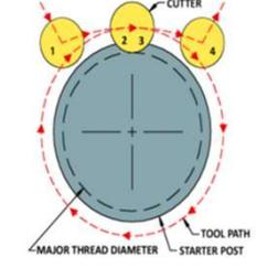
Step 1-2: Cutter engages part with arcing tool path while "Z" feeds down from top
