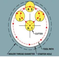
Step 1-2: Cutter moves into position
