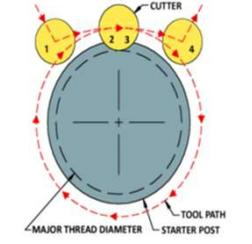
Step 1-2: Cutter engages part with arcing tool path while "Z" feeds up from bottom
