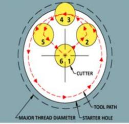
Step 1-2: Cutter moves into position
