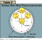
Step 1-2: Cutter moves into position Step 2-3: Cutter engages part with arcing tool path while "Z" feeds up from bottom
