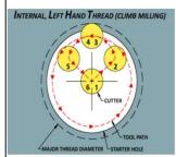
Step 1-2: Cutter moves into position Step 2-3: Cutter engages part with arcing tool path while <u>"Z" feeds down</u> from top
