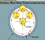
Step 1-2: Cutter moves into position Step 2-3: Cutter engages part with arcing tool path while "Z" feeds up from bottom
