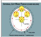
Step 1-2: Cutter moves into position Step 2-3: Cutter engages part with arcing from top
