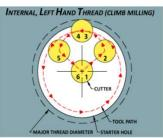
Step 1-2: Cutter moves into position
