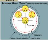
Step 1-2: Cutter moves into position Step 2-3: Cutter engages part with arcing tool path while "Z" feeds up
