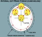
Step 1-2: Cutter moves into position Step 2-3: Cutter engages part with arcing tool nath while "7" feeds down from top
